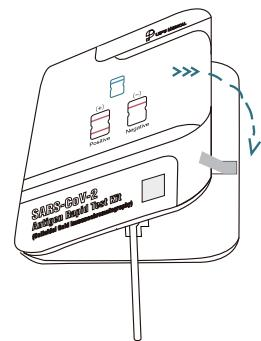
Step 4: Peel off the adhesive, fold the left side over, and wait for 15 minutes.
