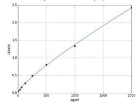
relative O.D.450 of each standard solution (Y) vs. the respective concentration of the standard solution (X). The Human TGF beta-1 concentration of the samples can be interpolated from the standard curve. If the samples measured were diluted, multiply the dilution factor to the concentrations from interpolation to obtain the concentration before dilution.
