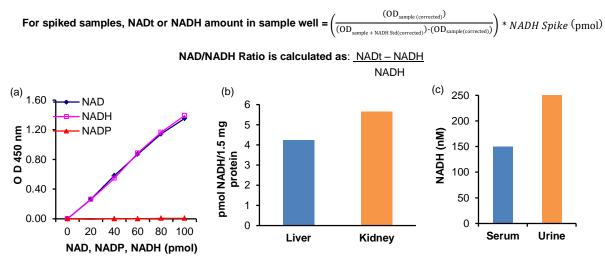
**Figure:** a) Standard Curve. b) Quantitation of NADH in rat liver (1.5 mg) and kidney (1.5 mg) homogenate. Tissues were washed with cold PBS followed by homogenization using NADH/NAD Extraction Buffer. Homogenates were centrifuged and deproteinized using a 10 kDa spin column (10000 x g, 10 min, 4°C). Filtrates were spiked with NADH (60 pmol) and assayed according to the protocol. (c) Quantitation of NADH in human serum (30 µl) and urine (30 µl).
