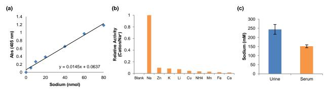
**Figure:** (a) Sodium Standard Curve. (b) Assay Specificity: Sodium, and other mono, di and trivalent cations (15 nmol/0.15 mM each) were tested to evaluate possible interferences. Interferences were found to be less than 10% when data was normalized using Sodium as 100% activity. (c) Estimation of sodium in human pooled serum Off-the-Clot (5  $\mu$ l; 50 times diluted), and human Urine (10  $\mu$ l; 100 times diluted). Assays were performed following the kit protocol.
