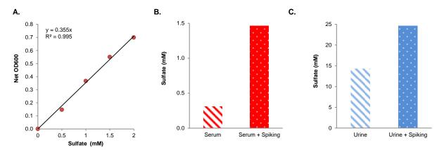
Figure A. Sulfate Standard Curve. Figures B Sulfate concentration determined in non-spiked and spiked (1.2 mM sulfate) serum samples C. Sulfate concentration determined in non-spiked and spiked (10 mM sulfate) urine samples. A spike recovery higher than 97% was obtained in both samples.
