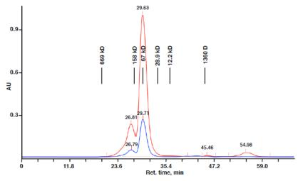
**Figure**: SEC chromatogram of BSA labeled with Cy5 using a Superdex 200 HR 10/30 column at 0.5 ml/min. in 50 mM Tris and 0.25 M NaCl pH 7.5. The absorbance was monitored at 280 nm (Blue line) and 650 nm (Red line). The spin column format ensured that the purification of protein was fast and there was no unreacted Cy5 left after the protein was purified according to the kit protocol.
