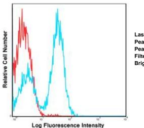
Laser: Blue (488nm) Peak Emission: 520nm Peak Excitation: 494nm Filter: 530/30 Brightness (1=dim, 5=brightest): 3
