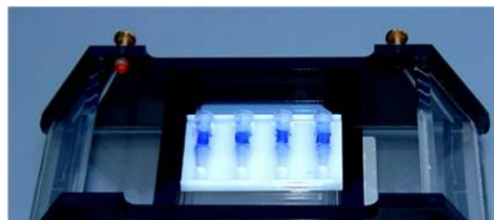
Figure 3: Supporting tray containing four DiaEasy™ Dialyzer tubes in a horizontal electrophoresis tank. The arrow on the cap is positioned face up and the two membranes of the DiaEasy™ Dialyzer tubes are in perpendicular to the electric field.
