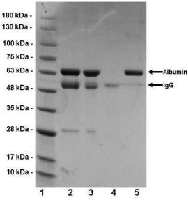
Figure: Hi-Bind<sup>™</sup> Albumin-IgG depletion beads were used to isolate human serum albumin HSA and IgG from a mixture of Human albumin and IgG (4-20% reduced SDS-PAGE):
