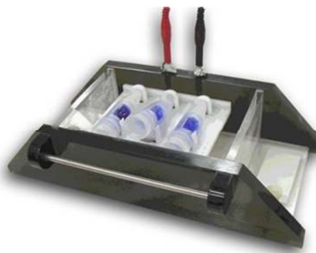
Figure 3: Supporting tray containing three DiaEasy™ Dialyzer tubes in a horizontal electrophoresis tank. The arrow on the cap is positioned face up and the two membranes of the DiaEasy™ Dialyzer tubes are in perpendicular to the electric field.
