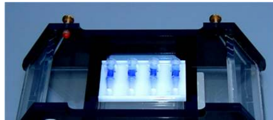
Figure 3: Supporting tray containing three DiaEasy™ Dialyzer tubes in a horizontal electrophoresis tank. The arrow on the cap is positioned face up and the two membranes of the DiaEasy™ Dialyzer tubes are in perpendicular to the electric field.
