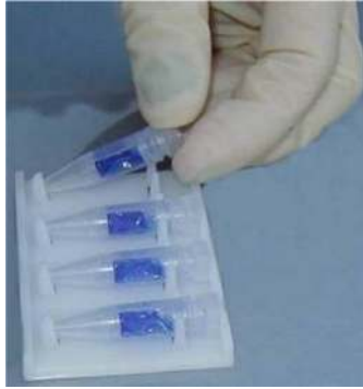
Figure 2: Insertion of the DiaEasy™ Dialyzer tubes in the provided supporting tray. The arrow on the cap is positioned face-up.
