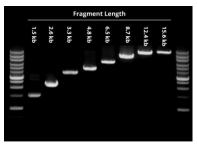
**Novo™ Reverse Transcriptase can elongate RNA templates up to 15 kb in length**. Novo™ Reverse Transcriptase was used in a reaction with a range of human RNA fragments. The resulting synthesized cDNA was followed by PCR and visualized on a 1% agarose gel.
