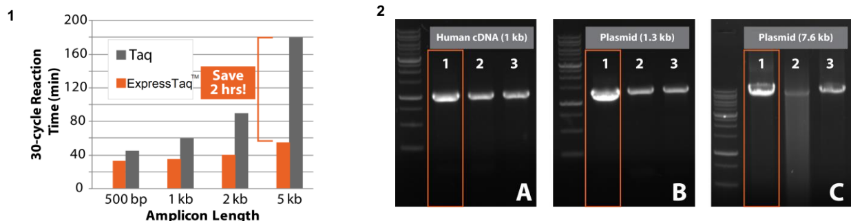
Fig 1. ExpressTaq™ DNA Polymerase enables extension speeds as fast as 6kb/min. Total reaction times for ExpressTaq™ DNA Polymerase and Taq Polymerase were determined for the amplification of different size amplicons: 500 bp, 1 kb, 2 kb and 5kb. Reaction
