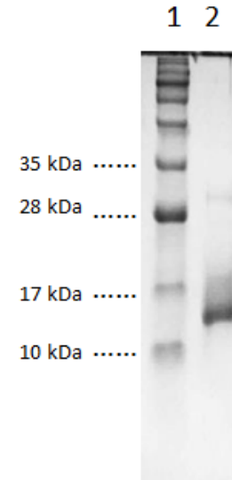
SDS-PAGE (12 %) of Human TGF- \beta 1: 1: Protein Marker 2: 5 \mu g Human TGF- \beta 1
