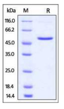
The purity of Human 4-1BB Ligand, Fc Tag was determined by SDS-PAGE under reducing condition and staining overnight with Coomassie Blue.
