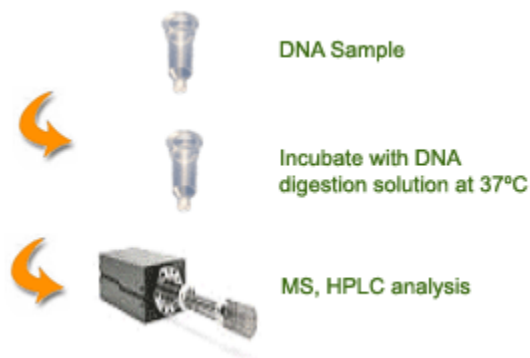
Schematic Procedure for Using the EpiQuik ™ One-Step DNA Hydrolysis Kit
