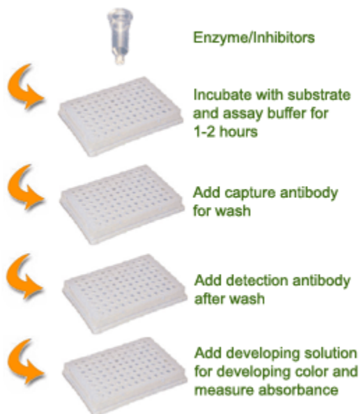
Schematic Procedure for Using the EpiQuik™ DNA Methyltransferase 1 Activity/Inhibitor Screening Assay Core Kit
